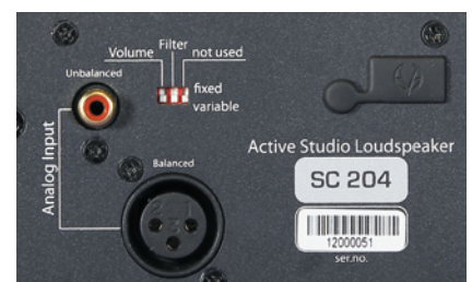
As well as the power and audio input sockets, the SC204's rear panel features DIP switches for locking various front-panel settings.
